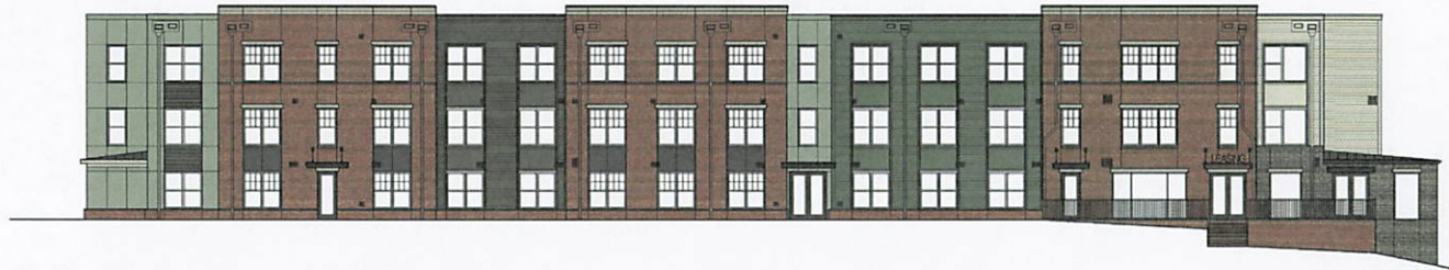
2 Building Type 1 North Elevation (Parking Lot Side) Scale: 1/8" = 1'-0" 1253 W. Oak Hill Ave. Type VA Construction 58% Brick
