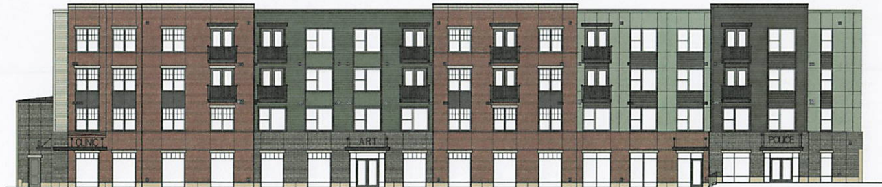
5 Building Type 1 West Oak Hill Avenue Elevation Scale: 1/8" = 1'-0" 1253 W. Oak Hill Ave. Type VA Construction 58% Brick
