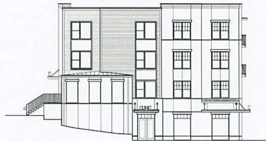
3 Building Type 1 West Elevation Scale: 1/8" = 1'-0" 1253 W. Oak Hill Ave. Type VA Construction 58% Brick
