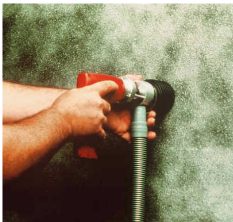
FIGURE 12.19 Needle Gun with HEPA Exhaust Ventilation.
