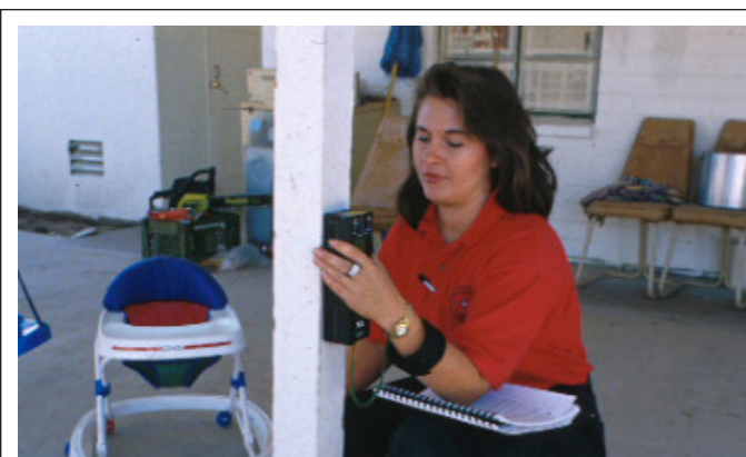
FIGURE 7.7 Lead inspectors should operate XRF instruments at a safe distance from others.
