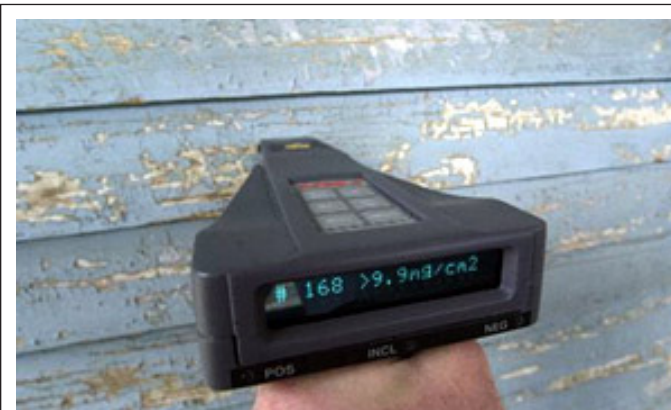
FIGURE 7.1 One type of XRF instrument displays its reading of a testing combination.
