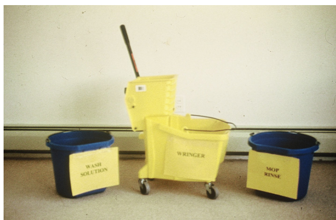
FIGURE 14.4 Three-bucket cleaning system.
