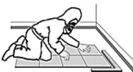
FIGURE 12.10 Install underlayment and new flooring as a suitable LBP enclosure method. The personal protective equipment is for a high-dust project.
