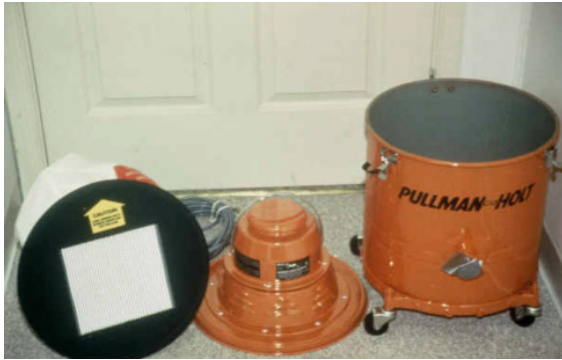
FIGURE 8.5 One example of a commercial-type HEPA vacuum.
